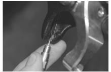
(12) Insert the throttle cable end into the finger lever slot.
