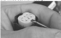
(7) Release the locking tabs holding the front cap on and pull the cap out until it stops. A second set of locking tabs prevent the cap from coming off completely.
