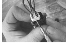
(6) Pull the rubber seal out and slide it back along the wires to give yourself enough room to pull the wires out individually.
