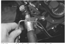
(11)Undo the clamp bolts on the Munster finger throttle using an Alan key. Route the wires from the heated grip through the open slot in the throttle block and clamp the finger throttle assembly to the handle bar. Re-route your throttle cable in front of your riser and handle bars. THE THROTTLE CABLE MUST BE AWAY FROM ANY PINCH POINTS. CHECK YOUR STEERING FOR FULL RANGE OF MOTION, MAKING SURE THERE IS NO STRESS OR TENSION ON THE CABLE HOUSING AT ANY POINT.
