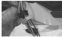
(15) Feed the finger heater wires through the plastic cap and rubber seal of the plug connector in any order. Plug the wires into the plug connector making sure the terminals are oriented in the right direction.
