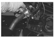
(19) Adjust and tighten kill switch if it was loosened. Adjust finger throttle placement for rider preference, and you're done!
