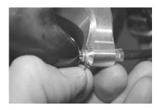
(14) Using the low profile C-clip provided with your finger throttle, install it over the end of the cable housing to secure it in place.
