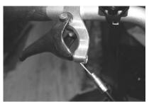
(13) Pull on the cable housing to extend the cable and insert the cable housing in the aluminum block.
