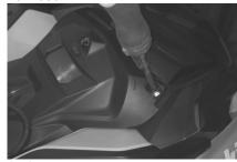
(10) Using zip ties, secure the wiring harness and any loose wiring to the machine. Re-install the hood and side panel, making sure to connect the air box and plug in any harness plugs you may have disconnected. Plug in and re-install the gauge, and you're done!
