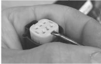
(5) Release the locking tabs holding the front cap on and pull the cap out until it stops. A second set of locking tabs prevent the cap from coming off completely.
