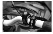
(7) Remove the clamp from the Munster kill switch with an Alan key and install the kill switch on the handle bar in your desired position. Route the kill switch wires through the wiring harness.
