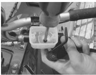
(5) Unscrew the Phillips screw inside the bottom of the reservoir.
