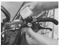
(6) Remove the plastic reservoir along with the rubber O-
