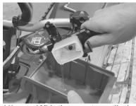
(4) With the master cylinder removed from the handle bar, dump out the fluid into a bucket and dispose of it.
