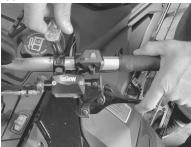
Pump the brake several times to allow any air bubbles to be removed from the master cylinder. Generally the system shouldn't need to be bleed unless the brake doesn't firm up after a few pumps. If the brake feels spongy at all after several pumps, you will have to bleed the brake system. Refer to your skidoo repair manual for proper brake bleeding procedure. ANY AIR IN YOUR BRAKE SYSTEM WILL CAUSE BRAKE FAILURE, DO NOT OPERATE YOUR MACHINE IF THE BRAKES ARE NOT WORKING PROPERLY. TAKE
