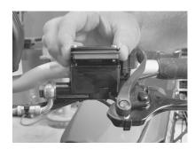
(11) Install the diaphragm and cap. Tighten down the cap bolts until you see the edge of the rubber diaphragm seal bulge only slightly. Do not overtighten, as it will squish the rubber diaphragm out of the flange and cause it to leak.
