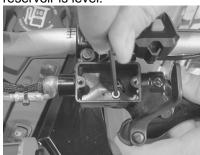
(9) Install and tighten the Allan screw included with your Munster brake reservoir. Only
