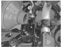
(10) Use DOT 4 brake fluid to fill the reservoir. Only fill the reservoir 80%, so that it doesn't overflow when you install the rubber diaphragm.
