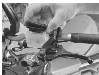
(2) Remove the cap and rubber diaphragm from the reservoir.
