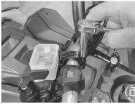
(3) Use an 8mm socket and rachet to remove the master cylinder bar clamp. Keep the master cylinder level so the fluid doesn't spill.
