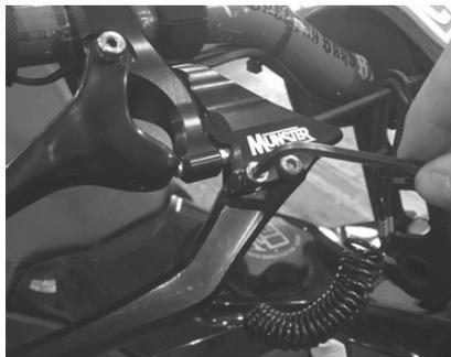
(4) Install the lever guard onto the guard body the same way you took it apart. Before you tighten the bolts fully, you can slide the lever side to side to adjust for rider preference. Tighten the bolts fully, making sure not to over tighten them and strip the threads.
