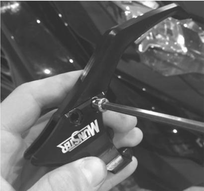
(1) After removing your throttle guard from the packaging, use an Alan key to remove the two bolts holding the throttle guard assembly together.
