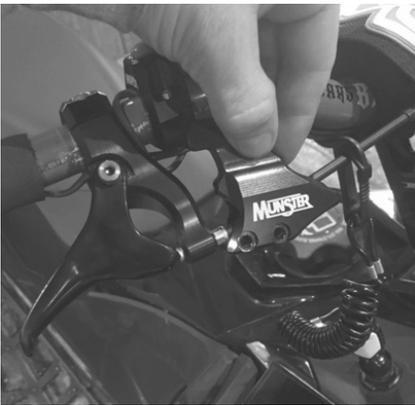
(2) Install the body of the throttle guard by sliding the throttle cable in the slot of the throttle guard body. Insert the two rounded mounting tabs into the sockets on the back side of your finger throttle.
